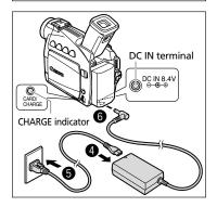
O The battery pack may be defective when the CHARGE indicator flashes rapidly.
